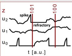
Stochastic comp. can naturally be implemented with spiking neurons by assigning refractory neurons the state  $z = 1$  and 0 otherwise.
