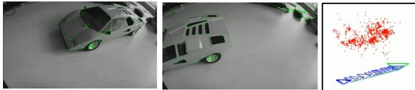
**Example of false start** (a case of consensus inversion) with ORB-SLAM 2 monocular. The camera is static and the car moves from right to left. **Left**: before car motion. **Middle**: after car motion. **Right**: final SLAM map (red) and computed poses (blue). The computed trajectory (right) is nonsense as there is no camera motion.
